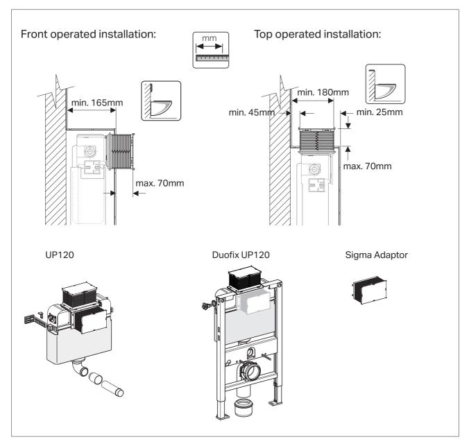
Please note: Cistern/Duofix must be installed in accordance to the drawing included in this document! Sigma50, Sigma20, Sigma01 and Bolero push-access plates only!
